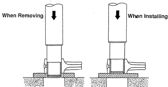
REPLACING THE SMALL END BUSHING
