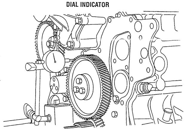
MEASURING GEAR SIDE CLEARANCE
