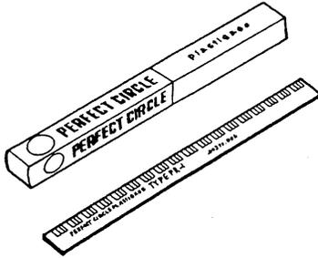
Application : Use to check the oil clearance between crankshaft and bearing, etc..
