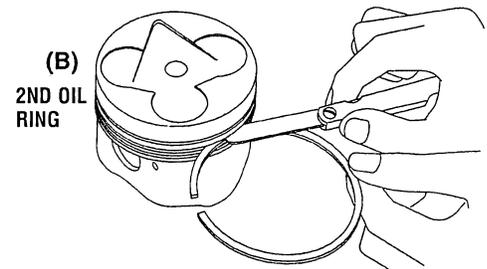
MEASURING THE PISTON RING CLEARANCE
