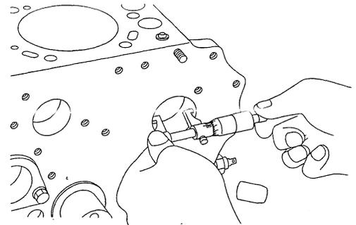
MEASURING THE CYLINDER BORE I.D.
