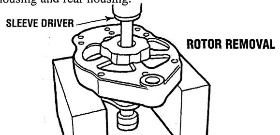
**NOTE:** If the bearing is removed from the housing, a new bearing must be installed.
