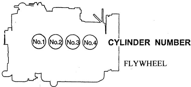
The sequence of cylinder numbers is given as No.1, No.2, No.3, and No.4 starting from the gear case side.
