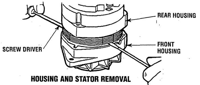
HOUSING AND STATOR REMOVAL
