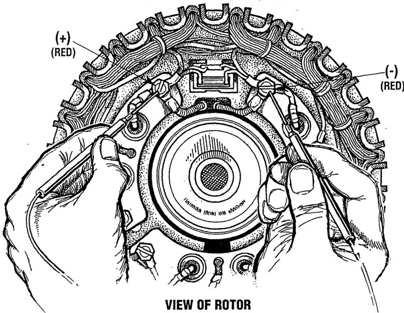
VIEW OF ROTOR FROM THE BEARING END
