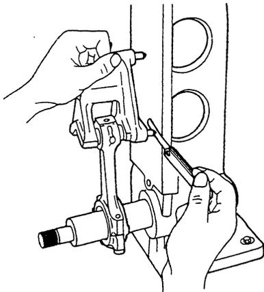
Application : Use to check the connecting rod alignment.
