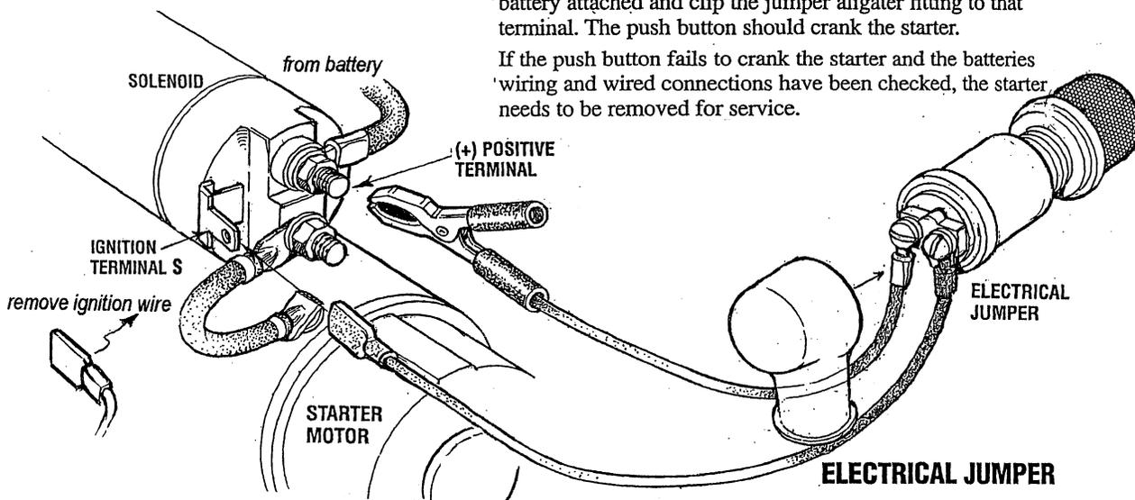
**NOTE:** This electrical jumper can be fabricated using a standard push button and two connecting wires.
